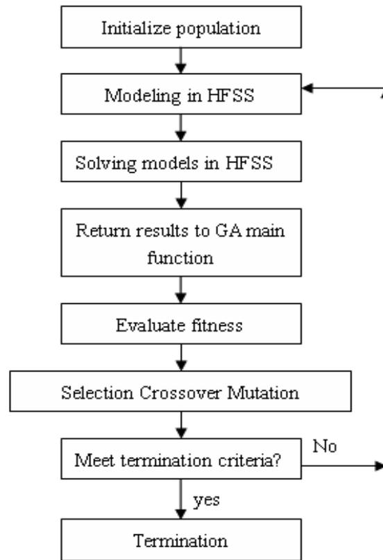
**Fig. 2** Flowchart representing HGA apply to micro strip patch.
