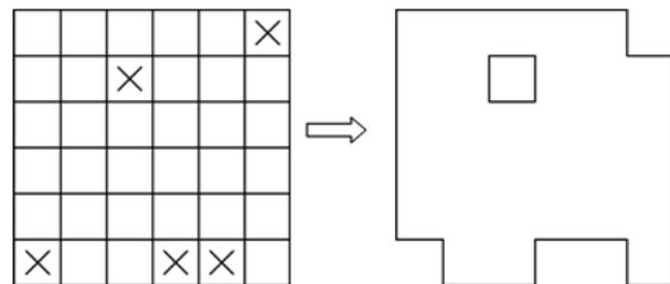
Fig. 1. Microstrip patch to be optimized.
